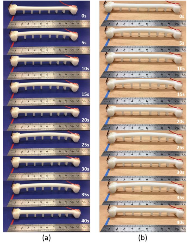
Fig. 9. Locomotion demonstration of proposed soft robot. (a) Locomotion on PP board. (b) Locomotion on wood board.
